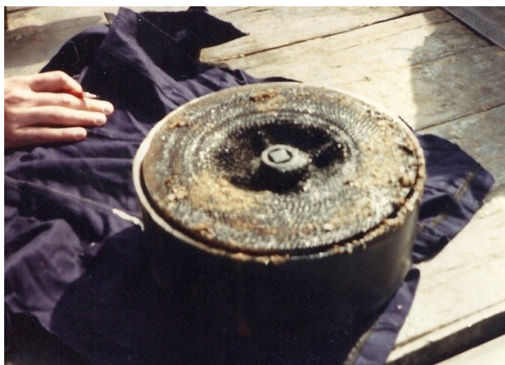
Figure 5. Historical photograph of a severely degraded flame-arrester element from the author's earlier field investigation material. It illustrates why condition of the element is part of the safety function. [1,8]
